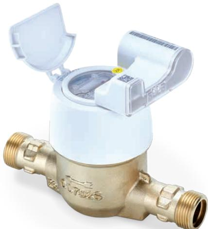
The **Electronic Data Capture** (EDC) module for non reactive, electronic pulse detection of all the ZENNER water meters whose registers are equipped with modulator disc enables a secure remote reading and the integration of water meters in Smart-Metering measurement systems.
